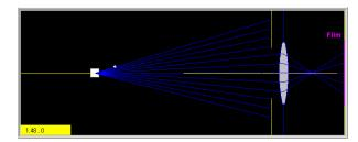
This animation can be used to demonstrate the basic operation of a camera (position is given in arbitrary units and angle is given in degrees). Various lenses and light sources can be added by clicking on the appropriate links. The camera is "focused" by dragging the lens to change the lens to film distance.
