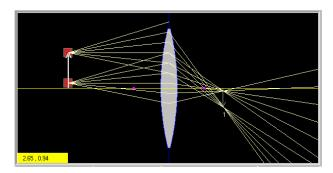
You will often use ray diagrams in order to determine where an image of an object will be, whether it will be real or virtual, and whether it will be inverted or upright (position is given in meters). The animation shows an object arrow, a lens, and pink dots to show the focal point of the lens. Restart.
