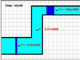
Bernoulli's equation describes the conservation of energy in an ideal fluid system. Assume an ideal fluid (**position is given in meters and pressure is given in pascals**). The dark blue in the animation is a section of water as it flows into the region marked by the horizontal line and the corresponding water that must move out of the region in the top right. We will explore the connection between Bernoulli's equation and conservation of energy. [Restart](#).
