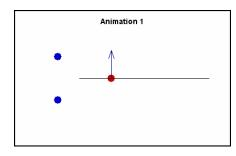
Each animation shows a positive charge (red) along with two unknown charges (blue). The electrical force on the positive charge is represented with a force vector. You can drag the red charge along a portion of the x axis (**position is given in meters and force is given in (newtons / k), where k is the constant in Coulomb's law)**.
