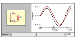
Assume an ideal power supply. The graph shows the voltage (red) as a function of time across the source and the current (black) through the circuit (voltage is given in volts, current is given in milliamperes, and time is given in seconds). (Note: the initial current versus time graphs are not centered about 0 because of the initial state of the capacitor and inductor.) Restart.
